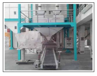
**PACKAGING SECTION** After grading we pack final rice in 5kg to 50kg packaging as per requirement .This machine is fully automatic
