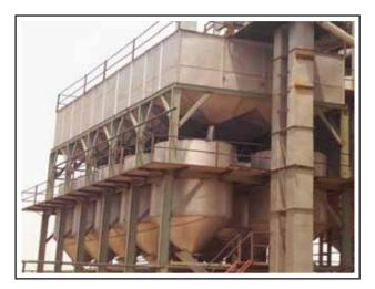
**PARBOILING AND STEAM PLANT** The process of parboiling uses processed soft water obtained from the water treatment plant.After parboiling we maintain the moisture using the dryer. We have three dryers, each with a capacity of 32 MT.
