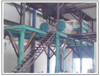
**PADDY CLEANER SECTION** We clean all extra particles like dust, paper, big size stones and wooden parts etc. The plant capacity is 20-25 MT per hour. After this we store clean paddy in silos.
